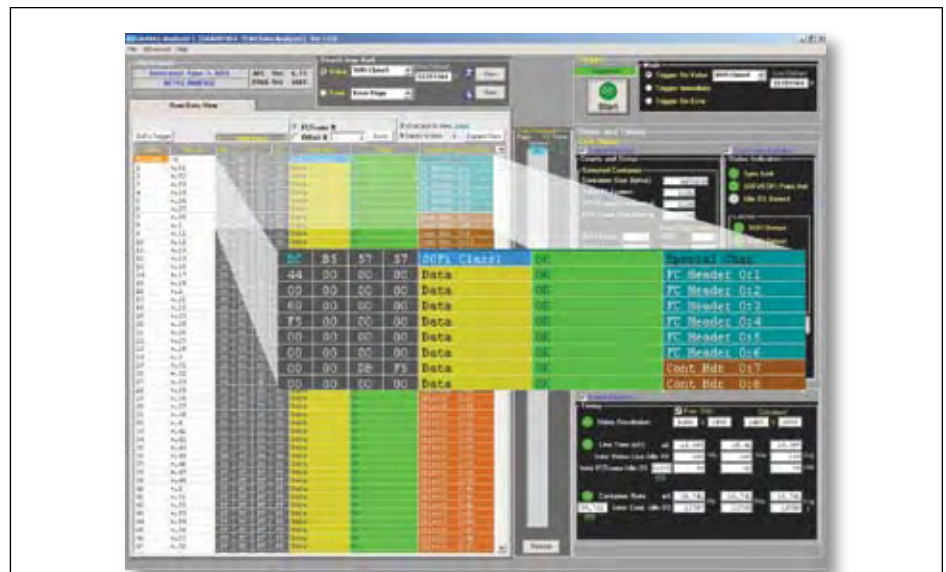
Figure 2 Data showing protocol trace is captured by Great River Technology's ARINC 818 protocol analyzer.
